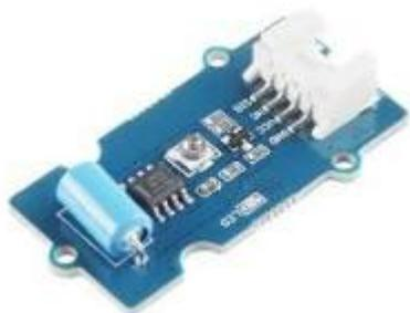
Vibration Sensor (SW-420) is a high sensitivity non-directional vibration sensor. When the module is stable, the circuit is turned on and the output is high. When the movement or vibration occurs, the circuit will be briefly disconnected and output low
